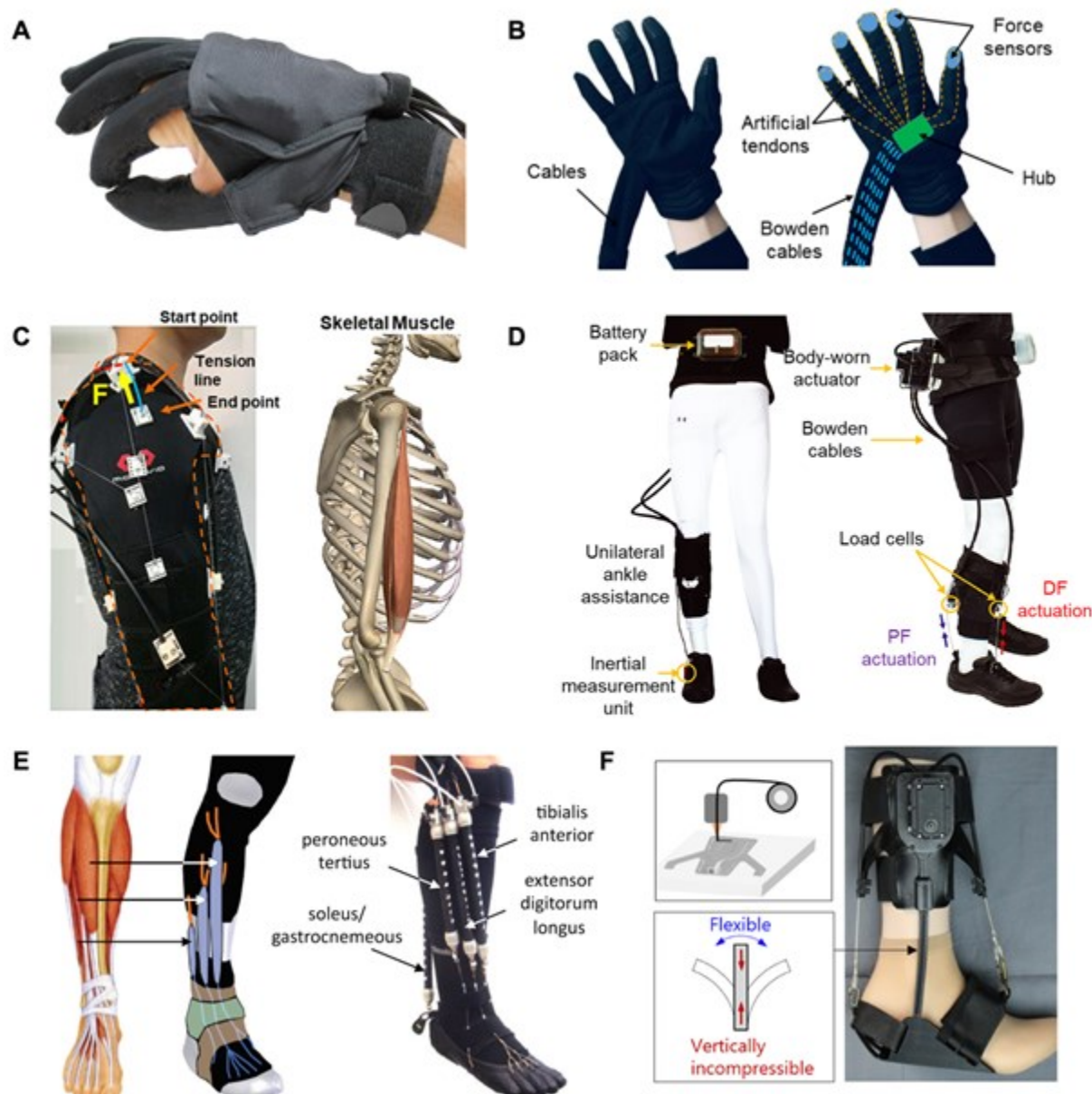
Figure 13. Soft actuators for disability rehabilitation. A) A pneumatic soft actuating glove for hand rehabilitation. Reproduced with permission. [394] Copyright 2016, IEEE. B) Motor glove with animation of tendon design for hand rehabilitation. Reproduced with permission. [158] Copyright 2021, IEEE. C) Bio-inspired soft exoskeleton for upper limb rehabilitation to reduce stroke-induced complications. Reproduced with permission. [493] Copyright 2021, IOP Publishing. D) Soft robotic exosuit for lower limb rehabilitation improves walking in patients after stroke. Reproduced with permission. [494] Copyright 2017, AAAS. E) Pneumatic soft wearable robotic device for ankle-foot rehabilitation. Reproduced with permission. [495] Copyright 2014, IOP Publishing. F) Soft wearable tendon-driven robotic ankle-foot-orthosis for post-stroke patients. Reproduced with permission. [496] Copyright 2019, IEEE.
